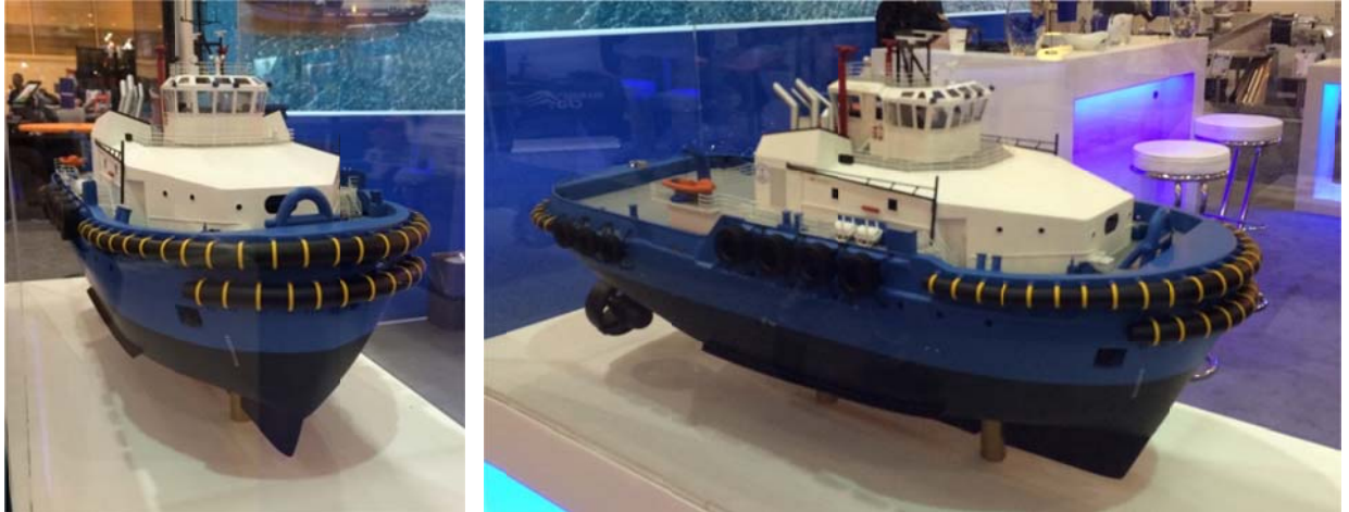
Figure 2 Model of Damen 4517 Tug, Indicating Bluff Forward Shape and Low Effective Bow Height to Bottom of Fenders (see also O/B Profile Drawing)
